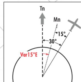
If the variation (Var) is to the East, it is subtracted from the geographical bearing to obtain the magnetic bearing. Ex.  $30^\circ - 15^\circ = 15^\circ$
