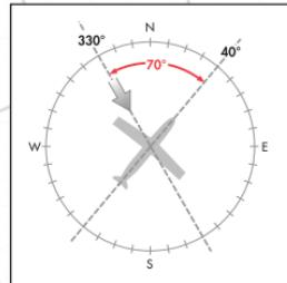
$$360^\circ - (330^\circ - 40^\circ) = 70^\circ \text{ (headwind)}$$
