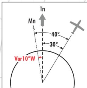
If the variation (Var) is to the West, it is added to the geographical bearing to obtain the magnetic bearing. Ex.  $30^\circ + 10^\circ = 40^\circ$
