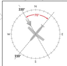
$$180^\circ - (330^\circ - 220^\circ) = 70^\circ \text{ (tailwind)}$$
