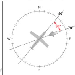
$$70^\circ - 40^\circ = 30^\circ \text{ (headwind)}$$
