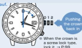
⚠ When the crown is a screw lock type, lock it. → P.99
